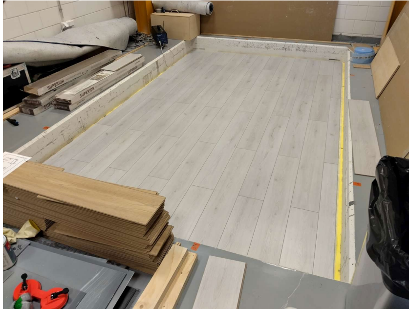
Figure A3.1. The specimens mounted on top of the reference slab in the test opening D. In the picture KronoTex Superior/Stella Advanced Laminate + KronoTex Basic plus sound proofing mat.
