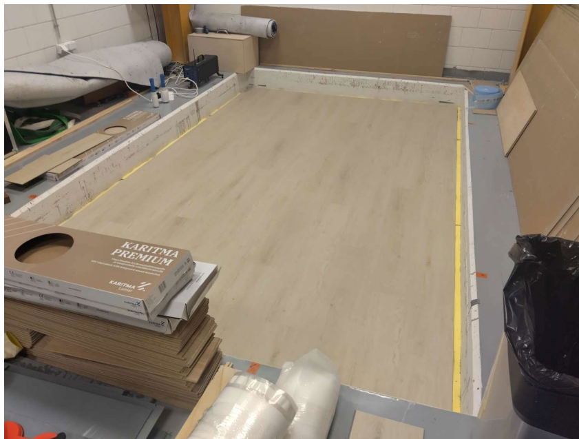
Figure A3.2. The specimens mounted on top of the reference slab in the test opening D. In the picture Karitma Premium Vinyl plank.
